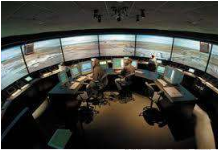
Fig 1.6-The 360 degree viewing screen in the NASA airport control tower simulator called the Future Flight Central Facility.
