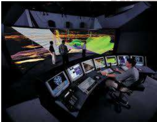
Fig 1.5-A geophysical visualization presented on a 25 foot semicircular screen, which provides a 160 degree horizontal and 40 degree vertical field of view.
