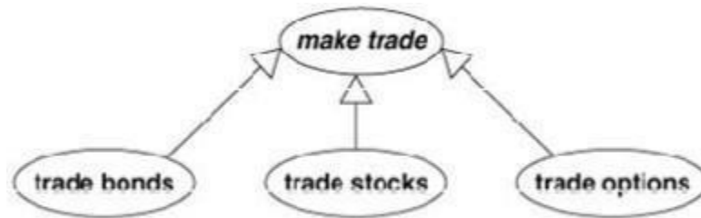
Figure 4.3 Use case generalization. A parent use case has common behavior and child use cases add variations, analogous to generalization among classes.
