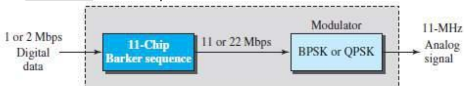
Figure 15.14 Physical layer of IEEE 802.11 DSSS
