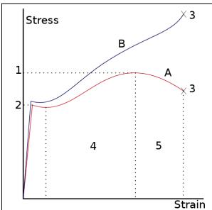
Stress—strain curve for low-carbon steel. Hooke's law is only valid for the portion of the curve between the origin and the yield point(2).
