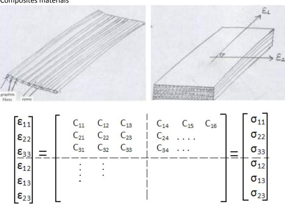
If there are axes of symmetry in 3 perpendicular directions, material is called **ORTHOTROPIC** materials.
