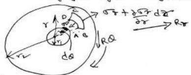
Rotational Symmetry: The stress distribution D symmetrical about wars of votables is called rotational Symmetry.
