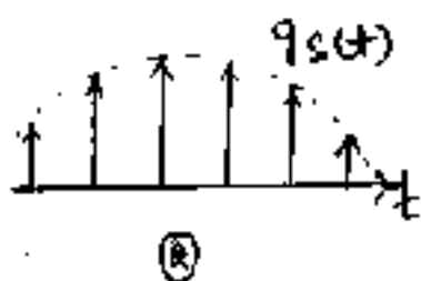
Fig : Recovering g(t) signal from sequence of samples g_s(t)
