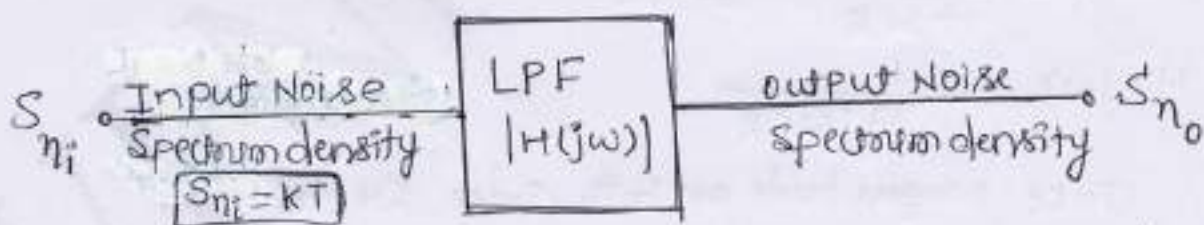
Fig 1: LPF with i/p & o/p spectral density
