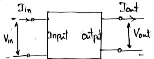
fig: Block diagram of amplifier showing input and output voltages and current.
