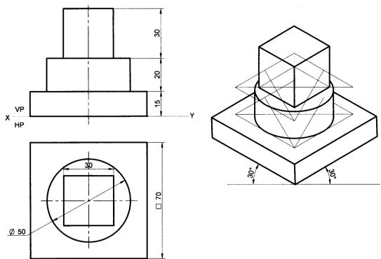
**Problem 32** Following figure shows the front and side views of solid. Draw the Isometric projection of the solid.
