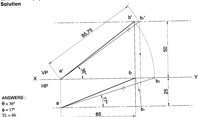
**Problem 45** A line has its end A, 15mm from HP & 10 mm from VP. The end B is 55mm from HP and the line is inclined at 30° to HP. The distance between the end projectors is 50mm. Draw the projections of the line. Determine the true length of the line and its inclination with VP.
