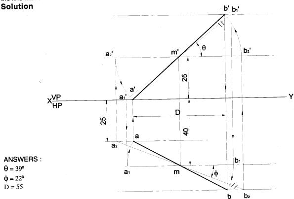
**Problem 44** The end A of a line AB is in HP and 25mm in front of VP. The end B is 25 mm infront of VP and 50mm above HP. The distance between the end projectors when measured parallel to the line of intersection of HP & VP is 65mm. Draw the projections of the line AB and determine its true length and true inclinations with HP & VP.
