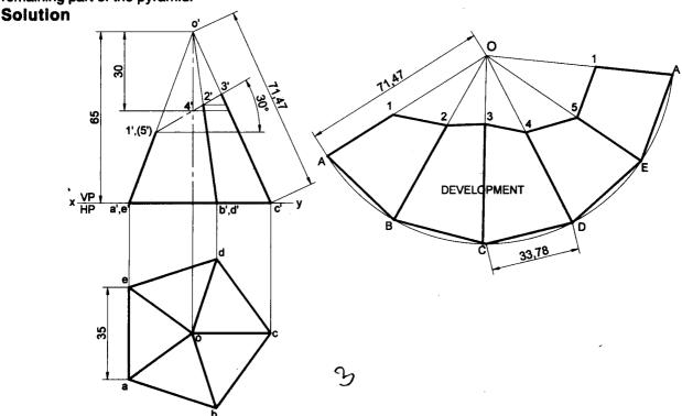
**Problem 25** A pentagonal pyramid, 30mm sides, with a side of base perpendicular to VP. Draw the development of the lateral surfaces of the retained portion of the pyramid shown by the dark lines in the following figure.
