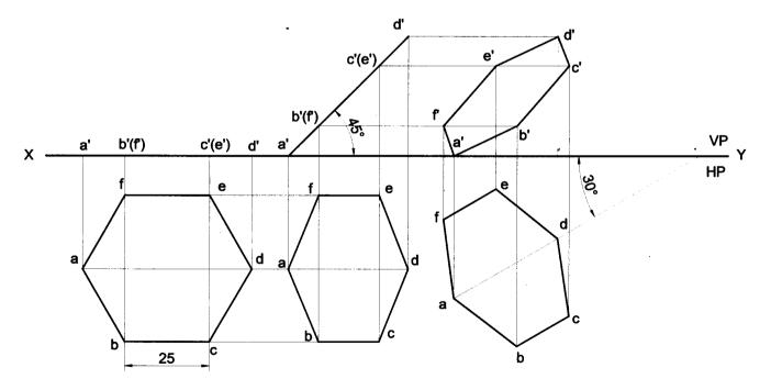
**Problem 43** A hexagonal lamina of sides 25mm rests on one of its sides on VP. The lamina makes 45° to VP and the side on which it rests makes 45° to HP. Draw its projections. **Solution**
