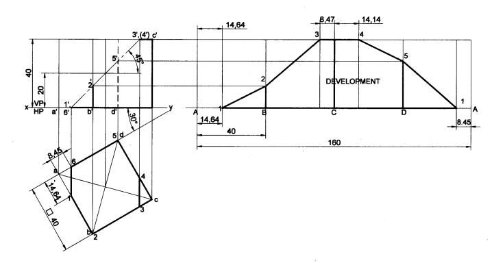
**Problem 6** A square prism of base side 35mm rests with its base on HP and two faces equally inclined to VP. Draw the development of the lateral surfaces of the retained portions of the cut prism shown by dark lines in the Fig. **Solution**
