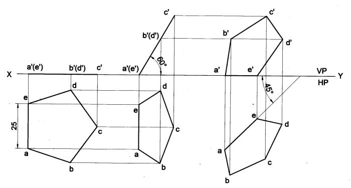
**Problem 20** A pentagonal lamina of edges 25mm is resting on HP with one of its corners such that the plane surface makes an angle of 60° with HP. The two of the edges containing the corner on which the lamia rests make equal inclinations with HP. When the edge opposite to this corner make an angle of 45° with VP and nearer to the observer, draw the top and front views of the plane lamina in this position.
