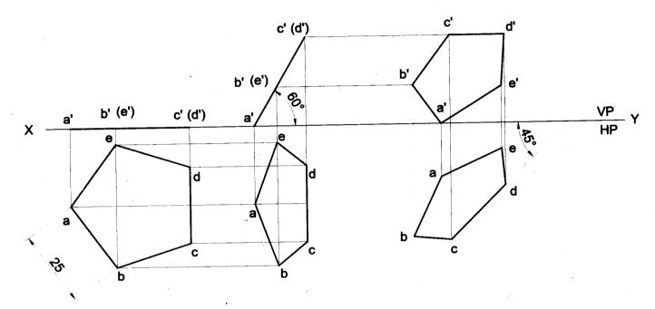
**Problem 21** A pentagonal lamina of edges 25mm is resting on HP with one of its corners such that the edge opposite to this corner is 20mm above HP & makes an angle of 45° with VP. Draw the top and front views of the plane lamina in this position. Determine the inclination of the lamina with HP.
