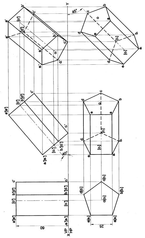
**Problem 8** A pentagonal prism 25 mm sides of base and 50 mm axis length rests on HP on one of its corners of the base such that the two base edges containing the corner on which it rests make equal inclinations with HP. Draw the projections of the prism when the axis of the prism is inclined to HP at 40° and to VP at 30°. **Solution**
