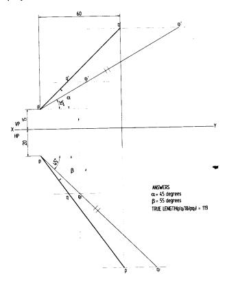
**Problem 32** The top view ab of a straight line AB is 60 mm long and makes an angle of 30<sup>0</sup> with the XY line. The end A is in VP and 30 mm above HP. The end B is 65 mm above HP. Draw the projections of the line AB and determine i) length of the front view ii) its true length and true inclinations with the reference planes.
