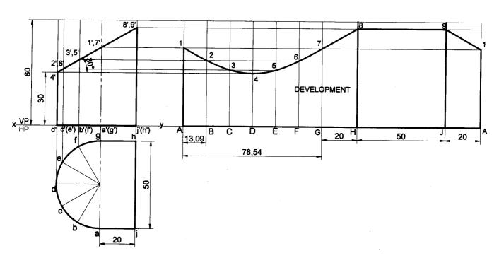
**Problem 35** Develop the lateral surface of the cylinder of 40mm diameter and height 60mm which is cut in the following way.
