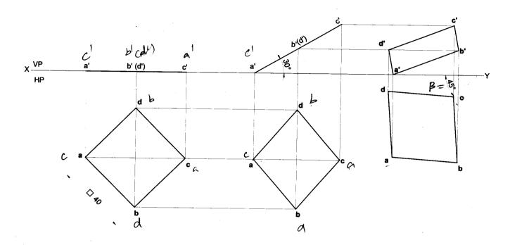
**Problem 11** The top view of a square lamia of side 30mm is a rectangle of sides 30mm x 20mm with the longer side of the rectangle being parallel to both HP and VP. Draw the top and front views of the square lamina. What is the inclination of the surface of the lamina with HP and VP? **Solution**
