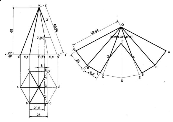
**Problem 30** A hexagonal pyramid of 30mm base sides with a side of base parallel to VP. Draw the development of the lateral surfaces of the retained portions of the pyramid cut by two perpendicular planes shown by dark lines in the Fig.
