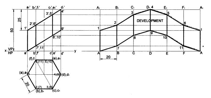
**Problem 16** A hexagonal prism of base side 25mm and height 55mm is resting on HP on its base, such that one of its base edges is parallel to VP. The prism is cut in this position as shown in the following front view. Draw the development of the lateral surface of the prism.
