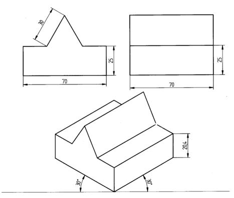
**Problem 45** A square prism of base side-30mm and length-70mm, is resting on its rectangular face on top of a square slab side -70mm and 25mm-thick. Draw the isometric projection of the combination
