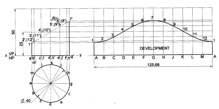
**Problem 40** Develop the lateral surface of the cylinder of 40mm diameter and height 60mm cut in the following way. **Solution**
