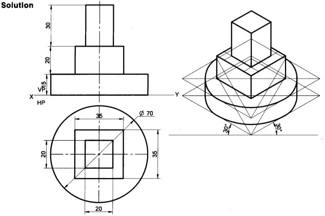
**Problem 31** Following figure shows the front and top views of solid. Draw the Isometric projection of the solid.
