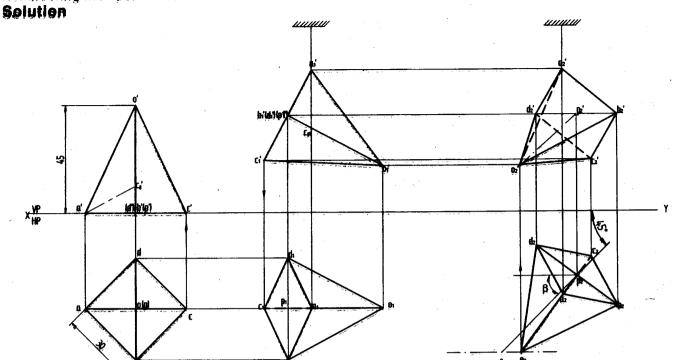
**Problem 50** A sone of base dia. 40 mm and axis length 50 mm is resting on HP on a point on the circumference of its base such that its apex is at 40 mm above the HP and its top view of the axis is inclined at 60° to VP. Draw the top and front views of the solid. Also, determine the inclinations of the axis when the base is nearer to the observer.
