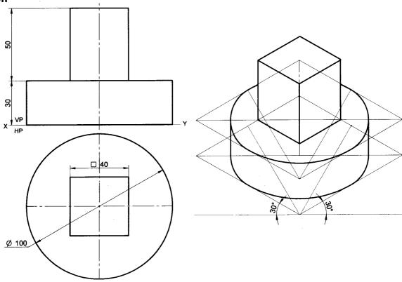
**Problem 21** A square prism base side-40mm, height50mm is placed centrally on a rectangular slab sides-100mmx60mm and thickness-20mm. Draw the isometric projection of the combination
