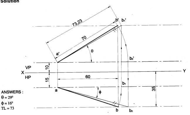
Problem 13 The distance between the end projectors through the end points of a line AB is 40 mm. The end A is 20 mm above HP and 15 mm in front VP. The end B is 45 mm infront of VP. The line AB appears 50 mm long in the front view. Complete the projections. Find the true length of the line and its inclinations with HP and VP. Solution
