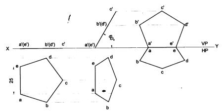
**Problem 25** A pentagonal lamina of sides 25mm is having a side both on HP and VP. The surface of the lamina is inclined at an angle of 60° with HP. Draw the top and front views of the lamina. **Solution**
