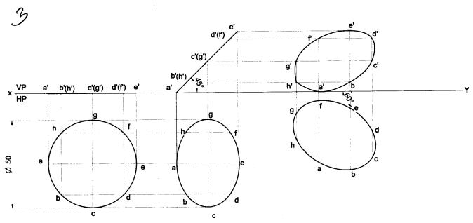
**Problem 47** A circular lamina of 50mm diameter is standing with one of its points on the rim on HP and the lamina inclined at 45° to HP. The diameter at right angles to the diameter which is passing through the point on which the lamina rests is parallel to VP. Draw its projections. **Solution**
