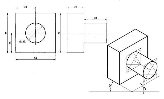
**Problem 30** Following figure shows the front and top views of solid. Draw the Isometric projection of the solid.
