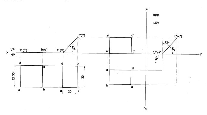
**Problem 12** A rectangular lamina of sides 20mm x 30mm rests on HP on one of its longer edges. The lamina is tilted about the edge on which it rests till its plane surface is inclined t HP at 45°. The edge on which it rests is inclined at 30° to VP. Draw the projections of the lamina.
