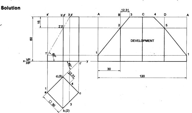
**Problem 3** A square prism of base side 40mm and axis length 65mm is resting on HP on its base with all the vertical faces being equally inclined to VP. It is cut by an inclined plane 60° to HP and perpendicular to VP and is passing through a point on the axis at a distance 15mm from the top face. Draw the development of the lower portion of the prism.
