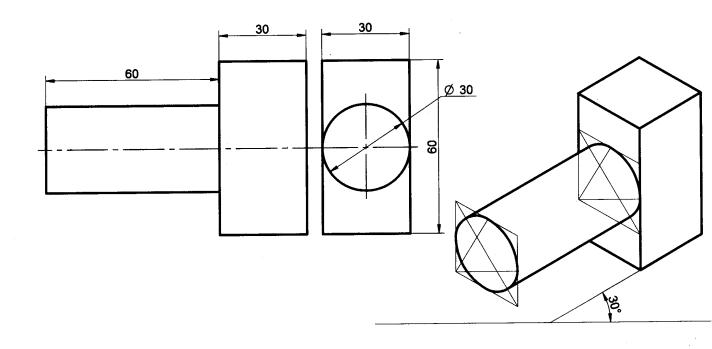
**Problem 29** Following figure shows the front and side views of solid. Draw the Isometric projection of the solid.
