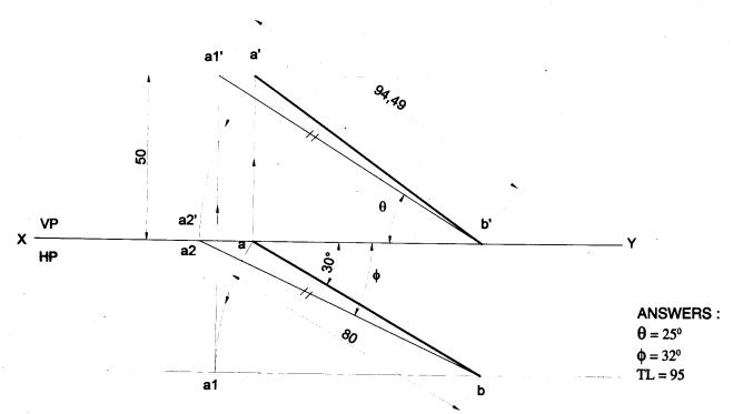
**Problem 15** Draw the projections of a straight line AB, 100 mm long, inclined at 45° to HP and 30° to VP. The end A is in HP and the end B is in VP. Find the shortest distance between the straight line AB and the line of intersection of planes of projection.
