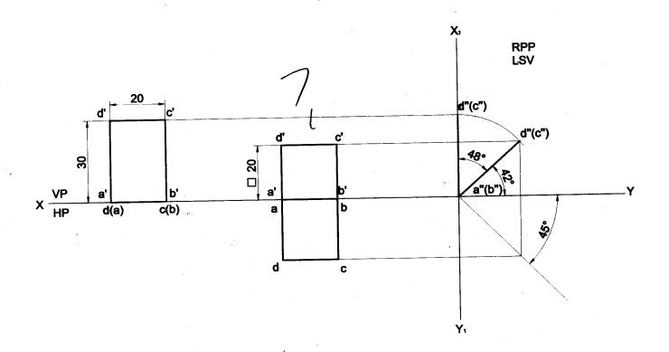
**Problem 17** A mirror 30mm x 40mm is inclined to the wall such that its front view is a square of 30mm side. The longer sides of the mirror appear perpendicular to both HP and VP. Find the inclination of the mirror with the wall.
