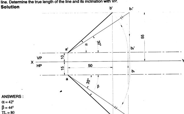
**Problem 8** The top view of a line 75 mm long measures 50 mm. the end P is 30 mm infront of VP and 15 mm above HP. The end Q is 15 mm infront of VP and above HP. Draw the projections of the line and find its true inclinations with
