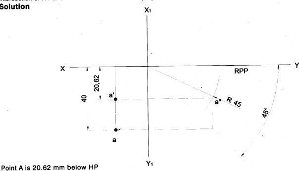
Problem 34 A point A is 20 mm above HP and in the first quadrant. Its shortest distance from the XY line is 40 mm .Draw the projections. Determine its distance from VP. Solution
