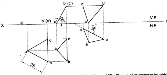
**Problem 5** A triangular plane lamina of sides 25mm is resting on HP with one of its corners touching it, such that the side opposite to the corner on which it rests is 15mm above HP and makes an angle of 30° with VP. Draw the top and front views in this position. Also determine the inclination of the lamina to the reference plane.
