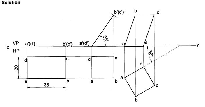
**Problem 15** A rectangular lamina of sides 20mm x 25mm has an edge in HP and adjoining edge in VP, is tilted such that the front view appears as a rectangle of 20mm x 15mm. The edge, which is in VP, is 30mm from the right profile plane. (a) Draw the top view, front view and the left profile view in this position. (b) Find its inclinations with the corresponding principal planes.
