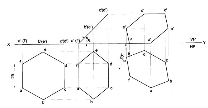
**Problem 41** A hexagonal lamina of sides 25mm rests on one of its corners on HP. The lamina makes 45° to HP and the diagonal passing through the corner on which it rests is inclined at 30° to VP. Draw its projections. **Solution**
