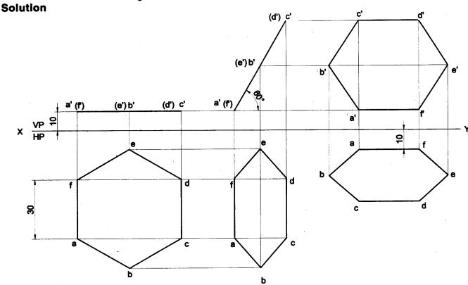
**Problem 34** A regular hexagonal lamina of sides 30mm is lying in such a way that one of its sides touches both the reference planes. If the lamina makes 60° with HP, draw the projections of the lamina.
