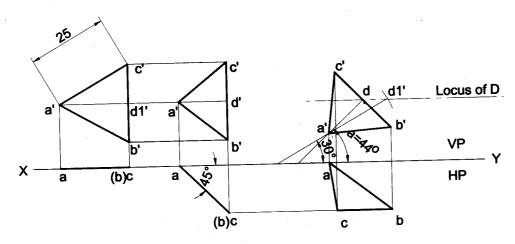
**Problem 4** A triangular plane figure of sides 25mm is resting on HP with one of its corners, such that the surface of the lamina makes an angle of 60° with HP. If the side opposite to the corner on which the lamina rests makes an angle of 30° with VP, draw the top and front views in this position.
