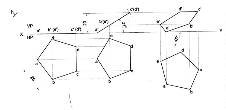
**Problem 22** A pentagonal lamina of sides 25mm is resting on one of its edges on HP with the corner opposite to that edge touching VP. This edge is parallel to VP and the corner, which touches VP, is at a height of 15mm above HP. Draw the projections of the lamina and determine the inclinations of the lamina with HP and VP and the distance at which the parallel edge lies from VP.
