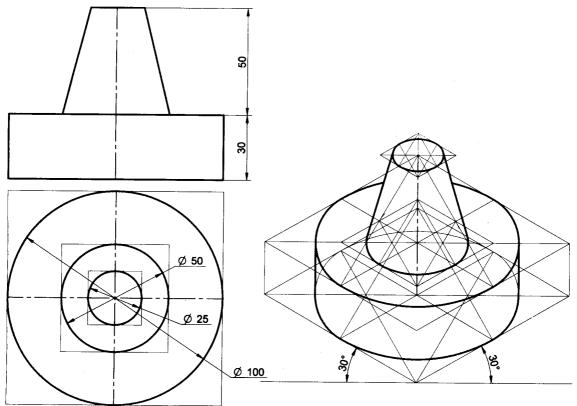
**Problem 23** A frustum of cone base diameter 50mm, top diameter 25mm and height 50mm is placed centrally on a square slab side-80mm and thickness-30mm. Draw the isometric projection of the combination.
