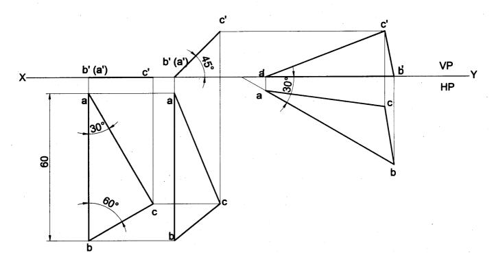
**Problem 7** An isosceles triangular plate of negligible thickness has base 25mm long and altitude 35mm. It is so placed on HP such that in the front view it is seen as an equilateral triangle of 25mm sides with the side that is parallel to VP is inclined at 45° to HP. Draw its top and front views. Also determine the inclination of the plate with the reference plane.
