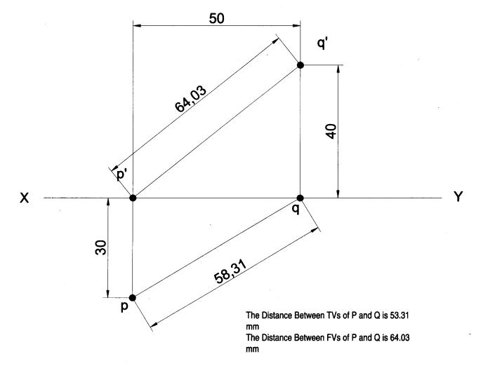
**Problem 15** A point P is 30 mm in front of VP, 40 mm above HP and 50 mm from RPP. Draw its projections. **Solution**
