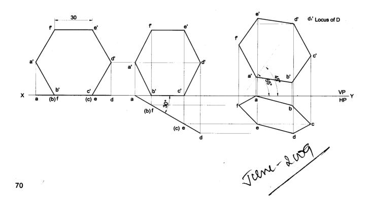
**Problem 39** A hexagonal lamina of sides 30mm is resting on HP with one of its corners in VP and its surface inclined at an angle of 30° with VP. The diagonal passing through that corner which is in VP appears to be inclined at 40° to HP. Draw the projections of the lamina.
