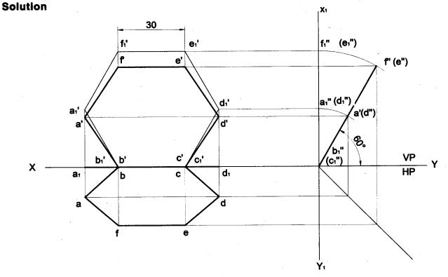
**Problem 35** A regular hexagonal lamina of side 30mm is lying in such a way that one of its sides touches both the reference planes. If the side opposite to the side on which it rests is 45mm above HP, draw the projections of the lamina.
