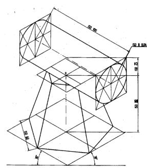
**Problem 5** Following figure shows the front view of combination of solids consisting a cut sphere and frustums of a cone and a square pyramid. Draw the Isometric projection of the combination of solids. **Solution**
