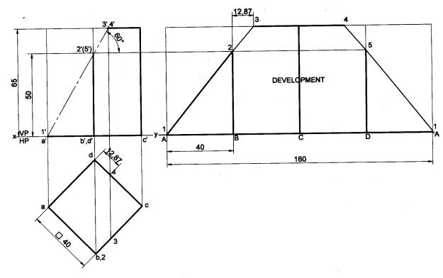
**Problem 4** A square prism of 30mm side of the base and height 50mm is resting with its base on HP such that one of its vertical faces is inclined at 40° to VP. It is cut as shown in the following front view figure. Draw the development of the lateral surface of the prism.
