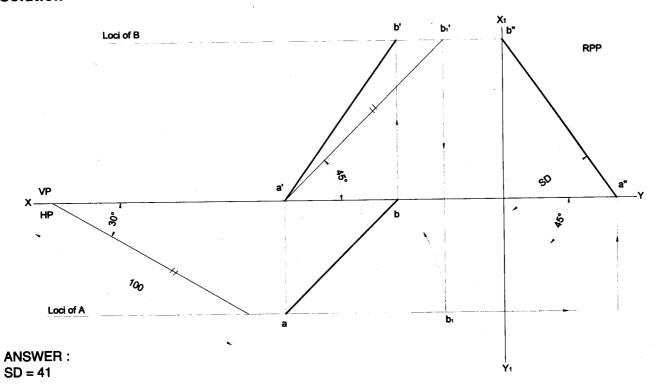
**Problem 16** A line AB 100 mm long is inclined to HP at 45° and inclined to VP at 30°. Draw front and top views of line and determine their lengths. Also determine the perpendicular distance of end Q from both HP and VP.
