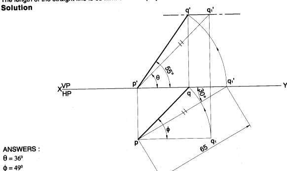
**Problem 37** Draw the projections of a line AB 90 mm long and find its true and apparent inclinations with HP and VP, when its end A is on HP and 20 mm in front of VP. Its midpoint M is 20 mm above the HP and 40 mm in front of the VP.
