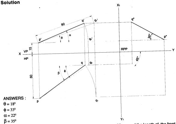
**Problem 48** The top view of a line AB, 80mm long measures 65mm and the length of the front view is 50mm. The end A is on HP and 15mm infront of VP. Draw the projections **Solution**
