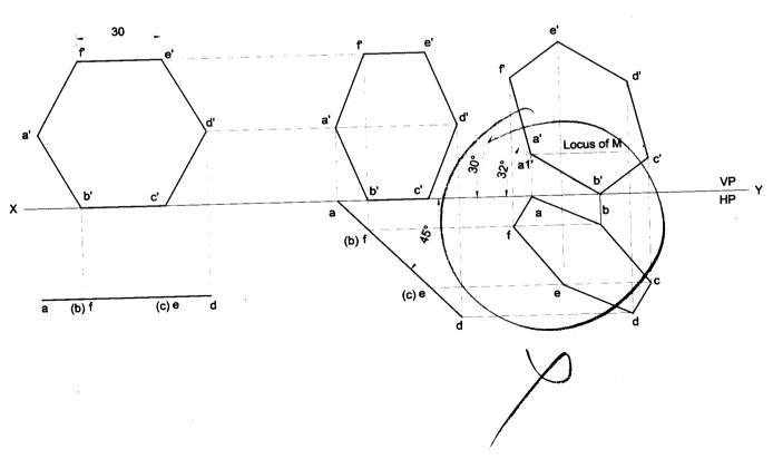
**Problem 33** Draw the top and front views of a hexagonal lamina of 30mm sides having two of its edges parallel to both vertical and horizontal planes and one of its edges is 10mm from each of the planes of projection. The surface of the lamina is inclined at an angle of 60° to the HP.
