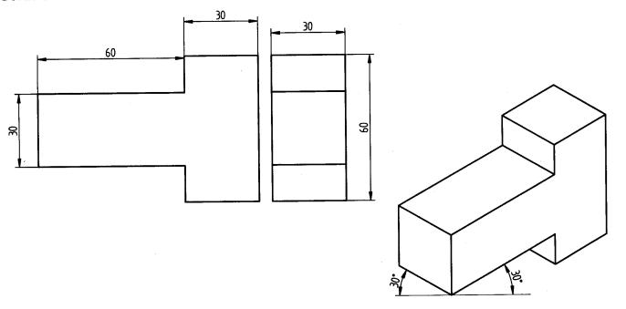
**Problem 28** Following figure shows the front and side views of solid. Draw the Isometric projection of the solid.
