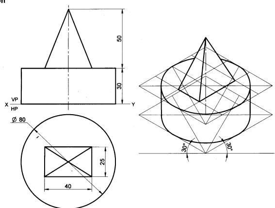
**Problem 19** A rectangular pyramid of base-40mmx25mm and height50mm is placed centrally on a rectangular slab sides-100mmx60mm and thickness-20mm. Draw the isometric projection of the combination
