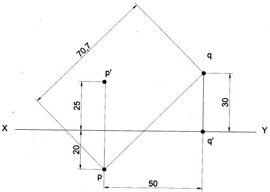
**Problem 37** A point A is on HP & 30 mm in front of VP. Another point B is 20 mm below HP and 20 mm in front of VP. The distance between their projectors measured parallel to XY line is 50 mm. Find the distance between the front views of the points A & B.
