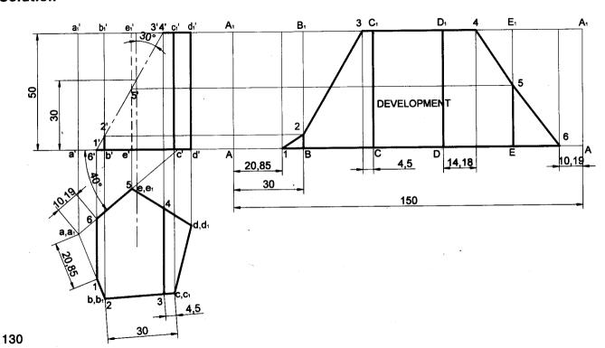
**Problem 13** A pentagonal prism of base sides 30mm and axis length 60mm rests with its base on HP and an edge of the base inclined at 45° to VP. It is cut by a plane perpendicular to VP, inclined at 40° to HP and passing through a point on the axis, at a distance of 30 mm from the base. Develop the remaining surfaces of the truncated prism.
