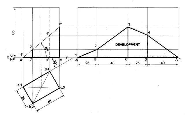
**Problem 10** Draw the development of the truncated portion of the lateral faces of a pentagonal prism of 20mm sides of base and 50mm height standing vertically with one of its rectangular faces parallel to VP and nearer to it so as to produce a one piece development. The inclined face of the truncated prism is 30° to its axis and passes through the right extreme comer of the top face of the prism. **Solution**
