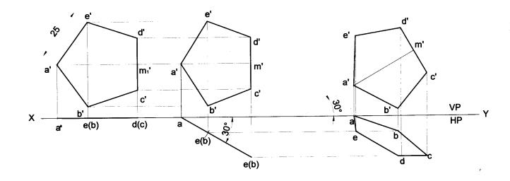
**Problem 31** A pentagonal lamina having edges 25mm is placed on one of its corners on VP such that the surface makes an angle 30° with VP and perpendicular bisector of the edge passing through the corner on which the lamina rests is inclined at 45° to HP. Draw the top and front views of the lamina.
