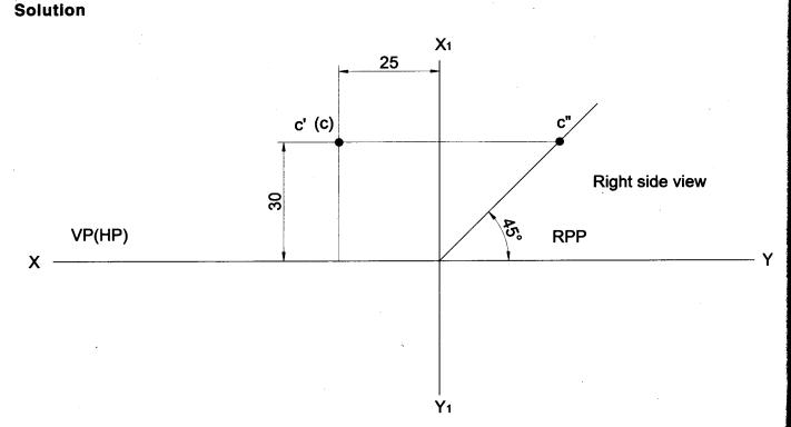
**Problem 45** A point is lying on VP, 10 mm below HP & 30 mm behind / in front / from LPP. Draw its projections and name the side view.
