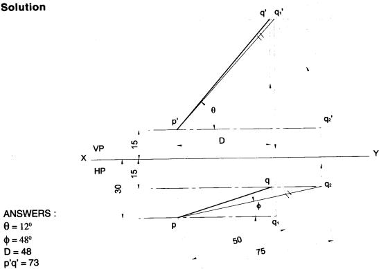
**Problem 28** A straight line AB measuring 80 mm long has the end A in the HP and 25 mm in front of the VP. Its mid point M is 25 mm above the HP and 40 mm in front of the VP. Draw the projections of the line and determine the inclination of the line with HP and VP.
