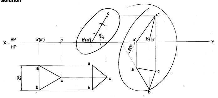
**Problem 2** An equilateral triangular lamia of 25mm side lies on one of its sides on HP. The lamina makes 45° with HP and one of its medians is inclined at 40° to VP. Draw its projections. **Solution**
