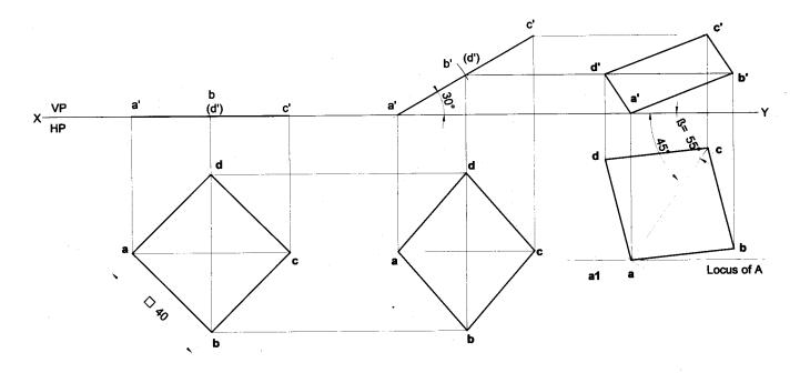
**Problem 10** A square lamia ABCD of 40mm side rests on corner C such that the diagonal AC appears to be at 45° to VP. The two sides BC and CD containing the corner C make equal inclinations with HP. The surface of the lamina makes 30° with HP. Draw its top and front views. **Solution**
