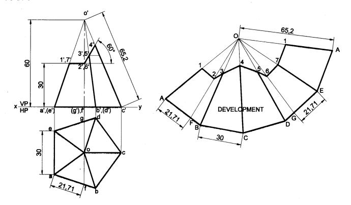
**Problem 26** A pentagonal pyramid of 30mm edges of base and 50mm height rests vertically with one of its base edges parallel to VP and nearer to it. It is cut as shown in following figure. Draw the development of the lateral surfaces of the upper portion of the pyramid.
