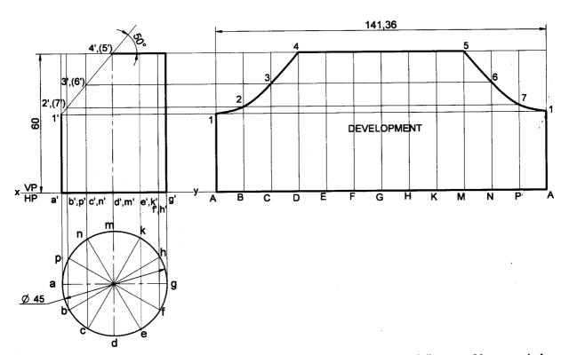
**Problem 32** Following figure shows the front view of a model of a steel chimney of diameter 60mm made from a flat thin sheet metal fitted over an inclined plane roof. Develop the portion of the chimney. **Solution**
