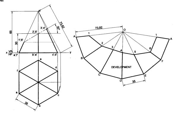
**Problem 29** A hexagonal pyramid 25 mm side of base and axis 65 mm long is resting on its base on HP with one of the edges of the base parallel to VP. It is cut by a vertical section plane at a distance of 8 mm from the axis towards right side. Develop the lateral surface of the left part of the pyramid.
