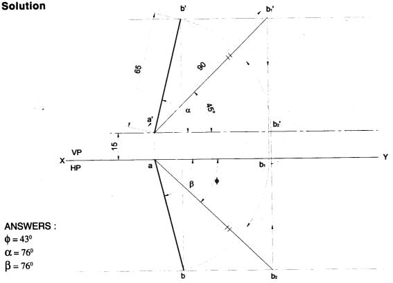
**Problem 12** The distance between the end projectors through the end points of a line AB is 60 mm. The end A is 10 mm above HP and 15 mm infront of VP. The end B is 35 mm infront of VP. The line AB appears 70 mm long in the front view. Complete the projections. Find the true length of the line and its inclinations with HP and VP. **Solution**
