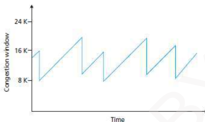
Figure 2.45: Additive-increase, multiplicative-decrease congestion-control
