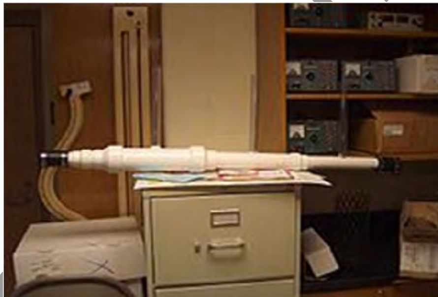
Fig. 2: Venturimeter - Experimental apparatus
