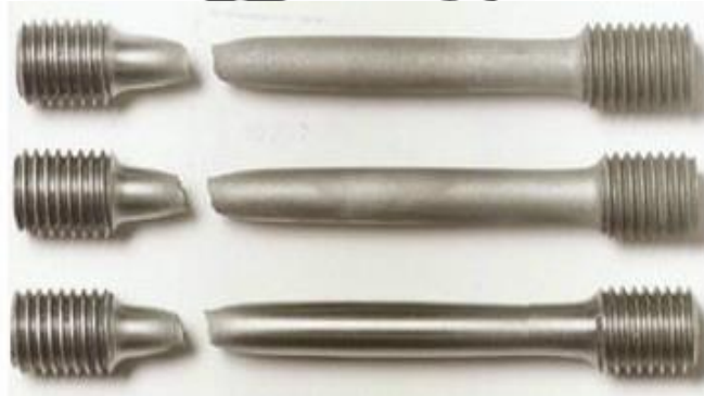
Necking in Tensile specimen
