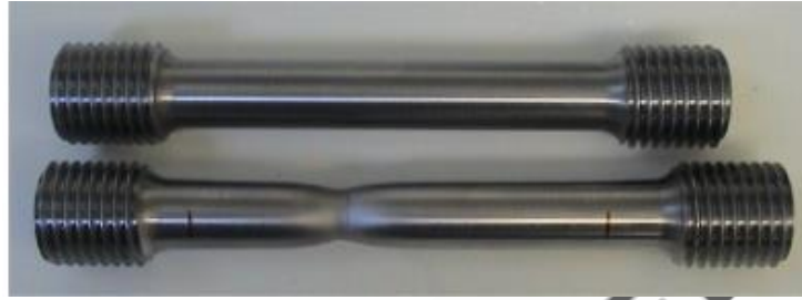
Necking in Tensile specimen
